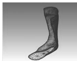
Fig.1 Shell model of PAFO
