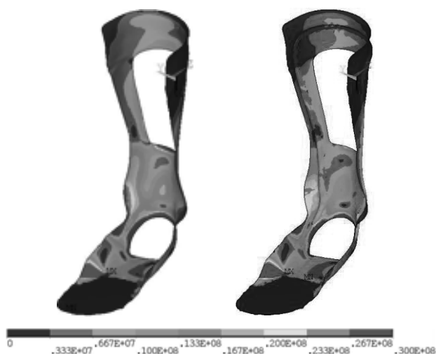
Fig.8 Quantity of equivalent stress distribution of dorsiflexion of patient.
