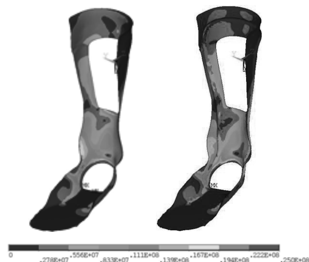
Fig.7 Quantity of equivalent stress distribution of plantar flexion of patient.
