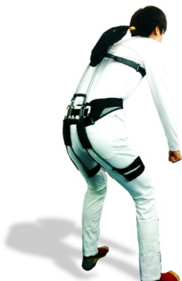
Assistance device for the lower back being developed by the author
